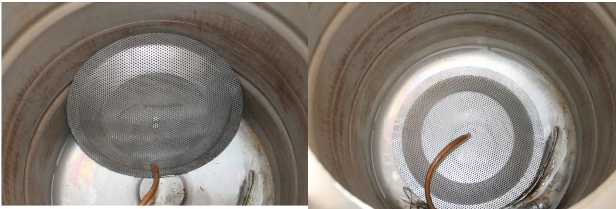
Screen laying in bottom of boil kettle and screen installed.
